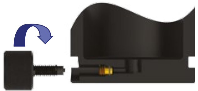
Discharge the gas spring with the vent key, pressing slightly on the valve.
