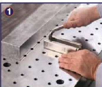
1 Bottom slide is made suitable to work piece and fixed.
