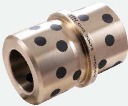
GRAPHITE / BRONZE GUIDE BUSH WITH CENTER COLLAR G. 45 DIN 9834 / ISO 9448 Self Lubricating
