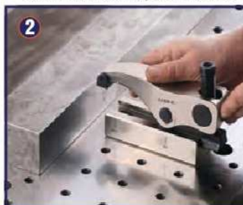
2 Upper casing is slid to slide, it is brought to position on work pieces.
