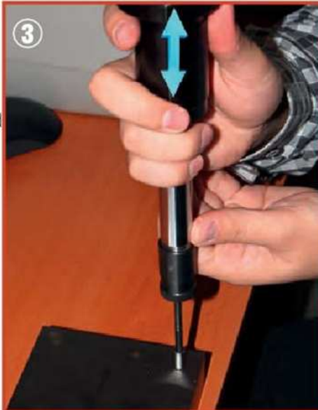
With a small impact application, pin is removed.
