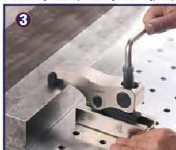
3 Fix upper bolt of lug to work piece.
